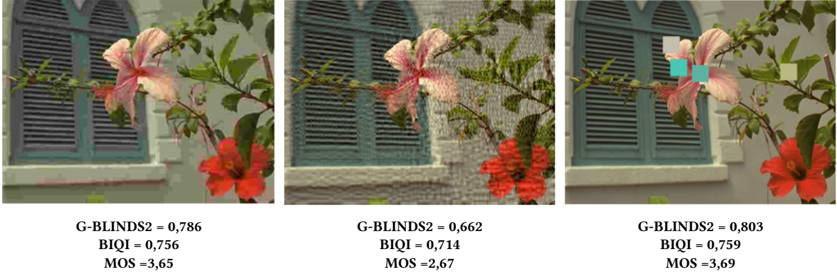
Figure 1: Examples of image quality scores performed using G-BLINDS2 and BIQI non-reference metrics.
